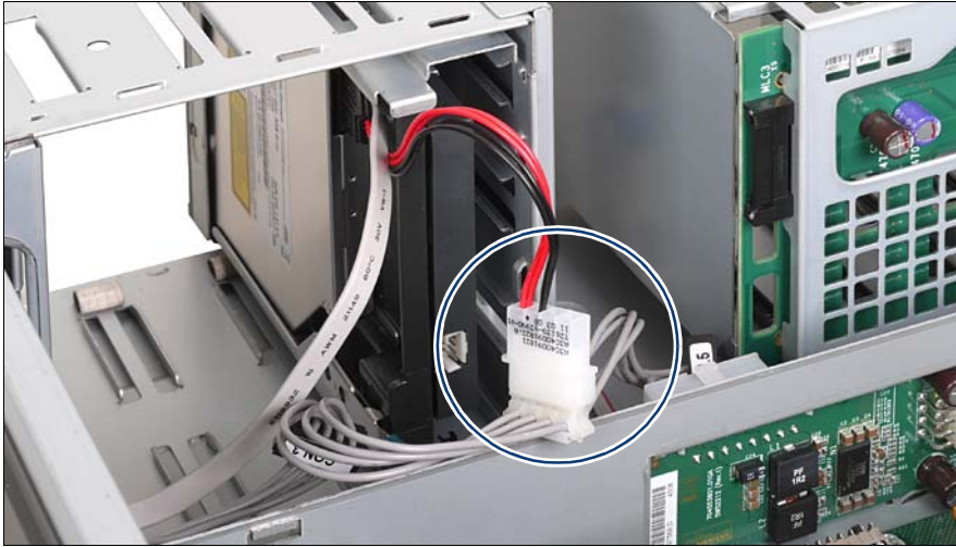
Figure 39: Connecting the PS adapter cable to the power cable
